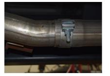
1. LAY OUT THE EXHAUST SYSTEM SO IT MATCHES THE DRAWING, MAKE SURE ALL PART NUMBERS ARE CORRECT. FOR AN EASIER REMOVAL OF THE FACTORY EXHAUST. CUT THE TAILPIPE JUST BEHIND THE FACTORY MUFFLER. LEAVE ALL RUBBER GROMMETS IN PLACE. USE WD-40 FOR EASIER REMOVAL OF FACTORY HANGER. UN BOLT THE FACTORY CLAMP LOCATED BEHIND THE FRONT RESONATOR AND **REMOVE MUFFLER AND** EXTENSION PIPE.
