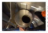
**3.** Next install the muffler by slipping it into the headpipe. Be sure the end marked "Inlet" is installed onto the headpipe. Rotate outlet to 4 o'clock position as seen in picture.
