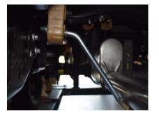
2. INSTALL HEADPIPE #A ONTO THE FACTORY PIPE. INSERT WELDED HANGER INTO RUBBER GROMMET. USE CLAMP #E TO ATTACH IT TO THE FACTORY PIPE. DO NOT TIGHTEN
