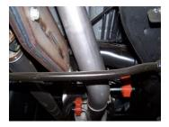
7. Install the over axle tailpipe #C into the extension pipe 1½-2". Use clamp #E to secure. Do not tighten. Insert welded hanger into the rubber grommet.
