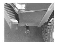
6. INSTALL THE STAINLESS TIP. ROTATE AND SLIDE TIP TO DEISRED LOCATION AND FIT. NOW TIGHTEN ALL CLAMPS, HANGERS, AND BOLTS.
