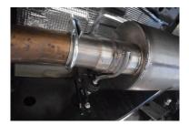
2. SLIDE MUFFLER ONTO THE HEADPIPE 1 <sup>1</sup>/<sub>2</sub>" TO 2". SO THAT THE LOCATOR PIN LOCATES INTO THE NTOCH ON THE MUFFLER ASSEMBLY. USE JACK STAND TO SUPPORT THE MUFFLER. ATTACH CLAMP #E AT THE INLET OF THE MUFFLER. THE MUFFLER OUTLET SHOULD BE POSITIONED AT ABOUT 1 O'CLOCK. DO NOT TIGHTEN
