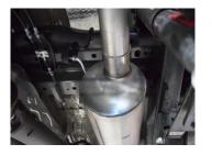
**4.** INSERT THE OVERAXLE TAILPIPE #B INTO THE OUTLET OF THE MUFFLER 1 ½" TO 2" INTO THE MUFFLER AND ATTACH USING CLAMP. INSERT WELDED HANGER INTO FACTORY RUBBER GROMMET. DO NOT TIGHTEN
