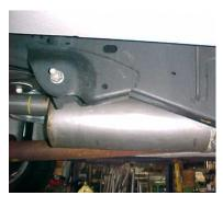
INSTALL MUFFLER # B ONTO HEADPIPE 1 ½" TO 2". USE CLAMP # E TO SECURE MUFFLER TO HEADPIPE. DO NOT TIGHTEN. USE A JACK STAND TO HOLD UP THE MUFFLER, MUFFLER INLET IS LOOKING INTO THE LOUVERS, OUTLET SHOULD BE AT THE 10 O'CLOCK POSITION.
