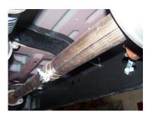
TO REMOVE YOUR STOCK EXHAUST, REMOVE IT FROM THE 2 BOLT FLANGE LOCATED JUST IN FRONT OF THE MUFFLER AND REMOVE
