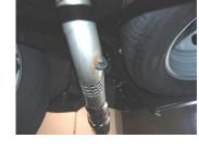
7. Adjust to fit properly then tighten all clamps and bolts. Use stainless steel cleaner to prevent tip from discoloration, Inspect all fasteners after 25-50 miles & retighten as necessary
