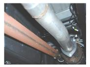
3.Disengage the welded hangers from the OEM rubber grommets. Use WD-40 to aid in the process. Do not damage or remove the rubber grommets as you will re-use them. Now, cut off tailpipe and remove exhaust. You also will re-use your factory nuts.
