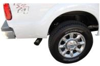
5. NOW INSTALL YOUR STAINLESS STEEL TIP. USE ANY ALUMINUM OR STAINLESS CLEANER TO POLISH YOUR TIP. THEN TIGHTEN ALL CLAMPS AND HANGERS.
