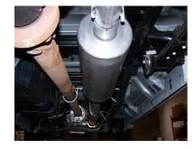
3. INSTALL MUFFLER # B. ONTO HEADPIPE 1½" TO 2". USE CLAMP #E TO SECURE MUFFLER TO HEADPIPE. DO NOT TIGHTEN
