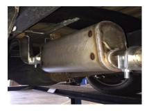
3. INSTALL MUFFLER # B. THROUGH BAND CLAMP THEN SLIDE ONTO HEADPIPE 1½" TO 2". USE CLAMP #E TO SECURE MUFFLER TO HEADPIPE.
