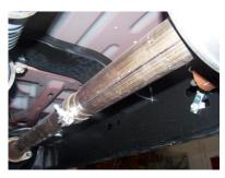
TO REMOVE YOUR STOCK EXHAUST, REMOVE IT FROM THE 2 BOLT FLANGE LOCATED JUST IN FRONT OF THE MUFFLER AND REMOVE HANGERS FROM RUBBER GROMMETS BY PULLING EXHAUST TOWARDS THE REAR OF THE VEHICLE, USE WD-40 TO AID IN REMOVAL, LEAVE GROMMETS IN PLACE.
