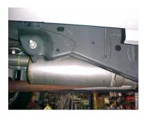
INSTALL MUFFLER # B ONTO HEADPIPE 1 ½" TO 2". USE CLAMP # E TO SECURE MUFFLER TO HEADPIPE. DO NOT TIGHTEN. USE A JACK STAND TO HOLD UP THE MUFFLER. MUFFLER INLET IS LOOKING INTO THE LOUVERS. OUTLET SHOULD BE AT THE 10 O'CLOCK POSTITON
