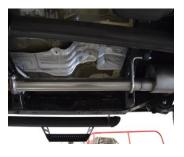
INSTALL HEAD PIPE #A ON TO YOUR EXISTING STOCK 2-BOLT FLANGE AND SECURE WITH BOLT KIT #F. INSERT WELDED HANGER INTO RUBBER GROMMET. DO NOT TIGHTEN
