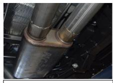
4. Install the Gibson Muffler with Logo facing downward. Use jackstand to support muffler Do not tighten until final install.
