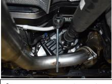
**3.** Install your Driver side head pipe #A using the factory Gasket and supplied bolts in Item #K and install your Passenger side headpipe. Do no tighten until final install.
