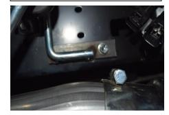
5. Install the hanger Item# I on the passenger side frame rail using the existing hardware that supported the OEM wiring harness bracket. Install rubber the hanger. Now Install the overaxle pipe into the outlet of the muffler. Note the long section of the pipe will go in the muffler outlet. Do not tighten.
