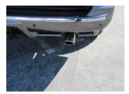
7. Install stainless steel tip. Clamp down. When you have everything in place, firmly tighten all bolts and clamps down securely. Use stainless steel cleaner and a Scotch Brite pad weekly to prevent tip from discoloration. Inspect all fasteners after 25-50 miles of operation and re-tighten as necessary.
