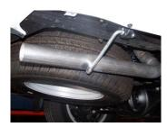
6. Install the exit pipe #D onto the tailpipe. Secure together with clamp #F. Do not tighten. Roll the exit pipe until it is at the correct angle for your vehicle. Insert welded hanger into rubber grommet.
