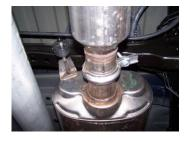
stem. Now, unbolt the ilpipe and remove exhaust. o not throw away stock inge bolts, as you will reuse em.
