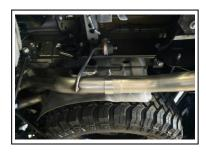
7. Lastly, install exit pipes (F) and tips (L) onto both Driver side and Passenger overaxle pipes. Position the exit pipes to what meets your expectations.
