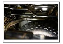
5. Continue by installing Passenger Side passenger over-axle pipe (D). Do not tighten using clamp #H to attach to muffler outlet.
