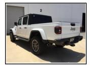
7. Install stainless steel tip onto the exit pipe to the desired length, and attach with bolt kit supplied. When you have everything in place, firmly tighten all bolts and clamps down securely. Use stainless steel cleaner weekly to prevent tip from discoloration. Inspect all clamps and bolts after 25-50 miles of operation and retighten as necessary.
