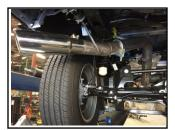
**6.** Remove the rear factory rubber insulator. Install the exit pipe #D onto the overaxle pipe and attach with band clamp# E. Re-install the factory rubber insulator. Do not tighten.
