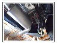
3. Install the Driver Side Muffler Assembly (Item B) by sliding the 2 1/2" Band Clamp (Item E) on the entrance of the assembly, installing the factory aluminum hanger on the assembly, and then sliding the entrance onto the left tube of the Y-Pipe. Return the factory hanger to its position with the factory hardware. Keep clamp and hanger loose.
