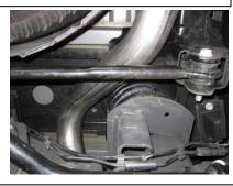
4. Install over axle pipe Item # B into the muffler outlet 1.5" to 2". Slip the hangers into the rubber grommets and keep tailpipe loose use clamp #c to secure together.
