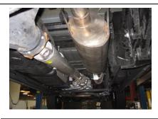
3. Install muffler assembly #A onto factory pipe insert hangers into rubber grommets use clamp #c to secure together do not tighten.
