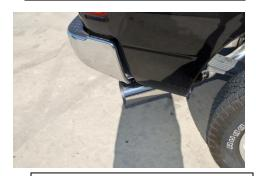
7. The system was designed to have the tip 1" below the quarter panel of the vehicle. With the tip in your desired position begin to tighten down all clamp connections from the front head pipe back. Clean tip before starting vehicle.
