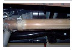
2. Install Item # A on to your factory exhaust using clamp # D to secure. Do not tighten.
