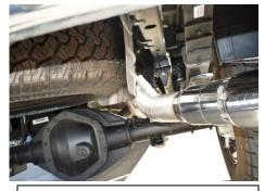
6. Install the exit pipe Item # B onto the over axle pipe. Do not tighten. Keep everything loose until you have proper clearance.
