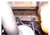
5. Next, install band clamp # F onto muffler, attaching with bolt kit #G. Insert hangers into rubber grommets. Do not tighten.
