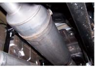
pipe #A 1 1/2"-2" with the louvers facing towards the converter. Use a jack stand to support the muffler. Use clamp #E to secure the muffler to the headpipe. Do not tighten. Muffler inlet is looking into the louvers. Outlet should be at the 10' O'clock position.
