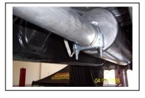
MAKE SURE YOU HAVE A 1" CLEARANCE ON ALL RUBBER BRAKE LINES, SHOCK BOOTS, TIRES, FUEL LINES, ETC..
