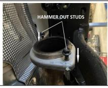
2. First you'll need to unbolt the factory flange and remove the exhaust. Next, hammer out the studs protruding from the factory flange, then install head pipe #A and tighten with allowance for adjustment using Bolt Kit #F
