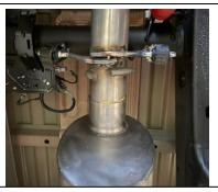
4. Slide the over axle tailpipe #C into the muffler 1.5-2". Use clamp #E to secure tailpipe to muffler. Do not tighten. Insert welded hangers into rubber grommets.
