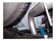
5. Slide the over axle tailpipe #C into the muffler 1.5-2". Use clamp #E to secure tailpipe to muffler. Do not tighten. Insert welded hangers into rubber grommets.
