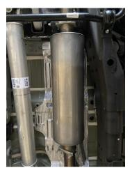
**4.** INSTALL MUFFLER #B ONTO HEADPIPE, USE CLAMP #D TO SECURE MUFFLER TO HEADPIPE. DO NOT TIGHTEN. USE A JACK STAND TO HOLD UP THE MUFFLER.
