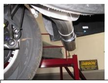
6. With proper clearance from spare tire install the exhaust tip onto the tailpipe. The system was designed to have the tip 1" below the quarter panel of the vehicle. With the tip in your desired position begin to tighten down all clamp connections from the front head pipe back.
