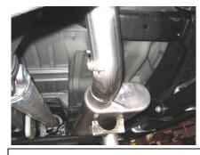
4. Install over axle pipe Item # C into the muffler outlet. Slip the hangers into the rubber grommets and keep tailpipe loose use clamp #E to secure together.
