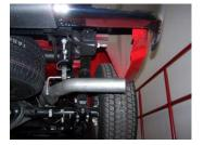
6. Slide exit pipe #D onto overaxle tailpipe using clamp #E to secure. Rotate exit pipe until it is at the correct angle for your truck. Insert welded hanger into rubber grommet.
