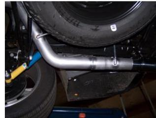
6. Install the overaxle tailpipe #D onto the intermediate tailpipe 1½"-2". Use clamp #G to secure pipes together. DO NOT TIGHTEN.
