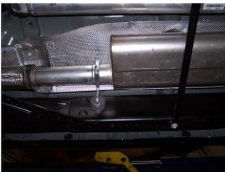
2. Install head pipe #A onto your existing stock flange and attach with factory hardware.
