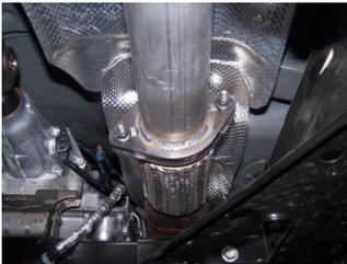
1. To remove the stock exhaust remove it from the flange located in front of your stock muffler. Disengage the welded hangers using WD-40 from the OEM rubber grommets. Do not damage or remove the rubber grommets as you will re-use them to mount your new system. Now, cut off tailpipe and remove exhaust.
