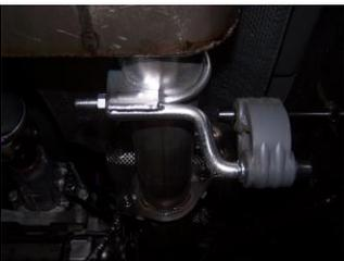
4. Install front muffler hanger #F onto inlet of the muffler. Insert welded hanger into rubber grommet. DO NOT TIGHTEN.
