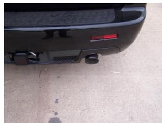
11. Install stainless steel tips. Clamp down. When you have everything in place, firmly tighten all bolts and clamps down securely. Use stainless steel cleaner and a Scotch Brite pad weekly to prevent tip from discoloration. Inspect all fasteners after 25-50 miles of operation and re-tighten as necessary.
