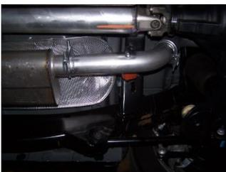
3. Install muffler #B onto head pipe #A 1½"-2". Use a jack stand to support the muffler. DO NOT TIGHTEN. Muffler outlet is looking into the louvers.
