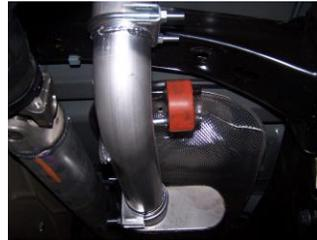
5. Install the intermediate tailpipe #C into the muffler 1½"-2". Use clamp #G to secure tailpipe to muffler. DO NOT TIGHTEN.
