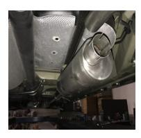
INSTALL MUFFLER # A ONTO HEADPIPE 1 ½" TO 2". USE CLAMP # F TO SECURE MUFFLER TO HEADPIPE. DO NOT TIGHTEN. USE A JACK STAND TO HOLD UP THE MUFFLER. OUTLET SHOULD BE CLOCKED AT 9 O'CLOCK
