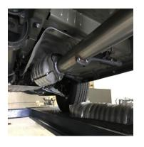
INSTALL HEADPIPE #B ONTO STOCK FLANGE. INSERT WELDED HANGERS INTO RUBBER GROMMET.
