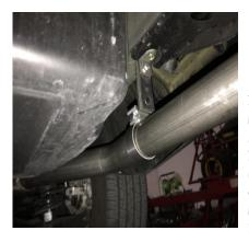
BOLT ON HANGER #E AS SEEN IN PHOTO AND USE CLAMP #F TO HOLD IN PLACE. INSTALL OVER AXLE PIPE ASSY # C INTO MUFFLER 1  $\frac{1}{2}$ " TO 2". INSERT HANGER INTO RUBBER GROMMET, USE CLAMP # F TO SECURE PIPE TO MUFFLER. DO NOT TIGHTEN.
