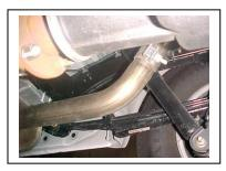
LAY OUT THE GIBSON EXHAUST ON THE FLOOR AND COMPARE PART #'S TO THE DRAWING. TO REMOVE YOUR FACTORY EXHAUST UN-BOLT YOUR TAILPIPE AT THE CLAMP LOCATED BEHIND YOUR STOCK MUFFLER USE WD-40 TO AID YOU IN REMOVAL OF HANGERS FROM RUBBER GROMMETS.
