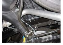
INSTALL THE OVERAXELE TAILPIPE #C INTO THE MUFFLER 1-1/2" TO 2". INSERT WELDED HANGERS INTO RUBBER GROMMET. SECURE TO THE MUFFLER USING CLAMP #E. DO NOT TIGHTEN.
