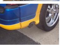
NEXT INSTALL YOUR STAINLESS STEEL TIP TO YOUR DESIRED LOOK. USE ANY ALUMINMUM OR STAINLESS STEEL CLEANER TO POLISH YOUR TIP. MAKE SURE YOU HAVE A MINIMUM OF A 1" CLEARANCE ON ALL PIPES FROM ALL RUBBER BRAKE LINES, TIRES, SHOCKS, FUEL LINES, ETC. THEN TIGHTEN ALL CLAMPS AND HANGERS
