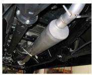
INSTALL MUFFLER #B ONTO HEAD PIPE 1-1/2" TO 2" WITH THE LOUVERS FACING TOWARDS THE CONVERTER. THE MUFFLER OUTLET SHOULD BE POSISTIONEDTHE MUFFLER OUTLET SHOULD BE POSITIONED AT 12:00. USE A JACK STAND TO SUPPORT TH E MUFFLER. USE CLAMP #E TO SECURE THE MUFFLER TO THE HEAD PIPE. DO NOT TIGHTEN. MUFFLER INLET IS LOOKING INTO THE LOUVERS.
