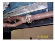
LAY OUT THE EXHAUST ON THE FLOOR SO IT LOOKS LIKE THE DRAWING AND COMPARE PARTS WITH MANUAL. TO REMOVE THE STOCK EXHAUST REMOVE IT FROM THE 2-BOLT FLANGE LOCATED IN THE FRONT OF THE MUFFLER. LEAVE ALL RUBBER GROMMETS IN PLACE. USE WD-40 TO AID IN REMOVAL OF EXHAUST AND HANGERS.
