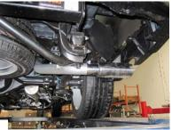
NEXT INSTALL REAR MUFFLER HANGER #G ONTO OUTLET OF MUFFLER. INSERT WELDED HANGER INTO RUBBER GROMMETS
