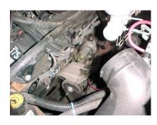
5. ON THE PASSENGER SIDE DISCONNECT THE DIP STICK FROM THE MANIFOLD, BUT DO NOT REMOVE IT. REMOVE THE MANIFOLD, SHIELD AND HARDWARE. CLEAN THE HEAD SURFACE WITH A WIRE BRUSH.
