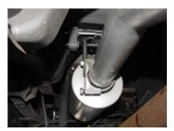
Install T-Hanger #E into factory rubber grommets in front of the muffler. **Do not tighten**
