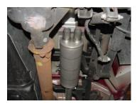
Slide muffler #B onto the head pipe with inlet towards the converter. Use a jack stand to support the muffler and clamp down using hanger #E. **Do not tighten**
