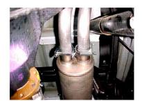
Clamps on muffler outlets should be positioned at 9 o'clock and 3 o'clock.
