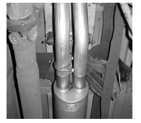
THEN, INSTALL DRIVERSIDE TAILPIPE #D. SUPPORT THE MUFFLER WITH A JACK STAND. THEN INSTALL PASSENGER SIDE OVERAXLE #C. INSERT WELDED HANGER ON TAILPIPE INTO FACTORY RUBBER GROMMENT. NOTE: SPARE TIRE MAY HAVE TO BE LOOSENED AND MOVED FOR BETTER CLEARANCES.
