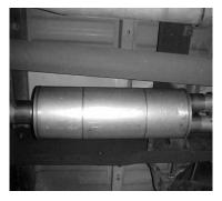
THEN INSTALL MUFFLER #B ONTO HEADPIPE #A AND CLAMP USING #F BUT DO NOT TIGHTEN. TO HELP SUPPORT YOUR MUFFLER, USE A JACK STAND. BEFORE INSTALLING OVERAXLE TAILPIPE, INSTALL REAR MUFFLER HANGER #E.
