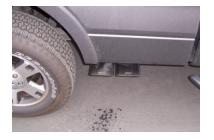
INSTALL STAINLESS TIPS, CLAMP DOWN. TO CLEAN YOUR STAINLESS TIPS USE ANY STAINLESS CLEANER OR A SCOTCH BRITE PAD. NOW GO AND TIGHTEN ALL CLAMPS, NUTS AND BOLTS. START FROM THE FRONT AND WORK BACK.
