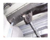
INSTALL WELDED HANGER INTO RUBBER GROMMET
