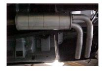
Install muffler assembly #A onto stock headpipe.
