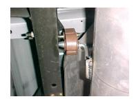
Install welded muffler hanger into rubber grommets.
