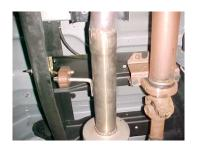
Install welded headpipe hanger into rubber grommet.
