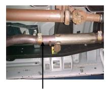
Then unclamp the second clamp before the muffler. Then cut tailpipe off just behind the muffler for easier removal.
