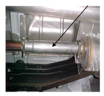
INSTALL NEW HEADPIPE # B AND ATTACH USING CLAMP # E TO FACTORY PIPE.
