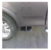
INSTALL THE STAINLESS STEEL TIP. USE ANY ALUMINUM OR STAINLESS STEEL CLEANER TO POLISH TIP. NOW TIGHTEN ALL CLAMPS AND BOLTS.
