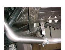
INSTALL PASSENGER SIDE OVERAXLE PIPE #C INTO MUFLER 1½" TO 2". USE CLAMP # I TO SECURE. DO NOT TIGHTEN. ROTATE UNTIL PIPE TOUCHES HANGER. #J USE CLAMP #I TO HOLD PIPE TO HANGER #J. DO NOT TIGHTEN.
