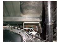
NEXT, LOCATE THE SLOTED HOLES LOCATED APPROXIMATELY 16" FROM THE REAR OF THE FRAME. MOUNT THE 10" STRAP HANGERS #J INTO THESE SLOTS USING THE HARDWARE PROVIDED. MOUNT USNG THE 2<sup>ND</sup> HOLE FROM THE TOP.
