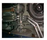
INSTALL DRIVERS SIDE TAILPIPE # D INTO MUFFLER 1  $\frac{1}{2}$ " TO 2". INSERT HANGERS INTO RUBBER GROMMETS, USE CLAMP # G TO SECURE PIPE TO MUFFLER. DO NOT TIGHTEN. THE TAB ON THIS PIPE SHOULD GO ON BOTTOM OF PASSENGER SIDE PIPE USE BOLT KIT # H TO SECURE TOGETHER.
