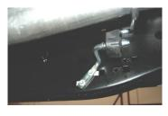
REMOVE THE HANGER FROM THE FRAME AND RELOCATE TO THE HOLES JUST TO THE LEFT OF THE OTHER HOLES. YOU WILL NEED TO PRY THE INSERTS OUT AND RE-INSTALL. SEE PHOTO.
