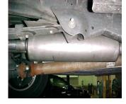
INSTALL MUFFLER # B ONTO HEADPIPE 1 ½" TO 2". USE CLAMP # F TO SECURE MUFFLER TO HEADPIPE. DO NOT TIGHTEN. USE A JACK STAND TO HOLD UP THE MUFFLER. DUTLETS SHOULD BE LEVEL.
