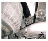
INSTALL PASS. SIDE TAILPIPE # C INTO MUFFLER 1  $\frac{1}{2}$ " TO 2". INSERT HANGER INTO RUBBER 9ROMMET, USE CLAMP # G TO SECURE PIPE TO MUFFLER. DO NOT TIGHTEN.
