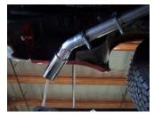
**7.** Next install the exit pipes #E. Use clamp #H, rotate pipes to the side. Trim ends of exitpipe to best fit your vehicle.
