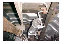
INSTALL HEADPIPE # A ONTO FACTORY PIPE. LINE UP THE NOTCH. USE CLAMP # H TO SECURE HEADPIPE TO FACTORY PIPE. DO NOT TIGHTEN. NEXT INSTALL FRONT MUFFLER HANGER #F ONTO HEADPIPE. SLIDE WELDED HANGER INTO RUBBER GROMMET. USE THIS CLAMP TO SECURE MUFFLER TO HEADPIPE. DO NOT TIGHTEN.
