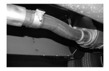
TO REMOVE YOUR STOCK EXHAUST, UNBOLT AND REMOVE THE CLAMP LOCATED JUST IN FRONT OF THE MUFFLER. FOR EASIER REMOVAL OF THE FACTORY EXHAUST, CUT OFF THE STOCK TAILPIPE JUST BEHIND THE MUFFLER AND REMOVE. LEAVE ALL RUBBER GROMMETS ON THE HANGERS. USE WD-40 TO AID IN REMOVAL OF EXHAUST AND HANGERS.
