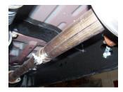
TO REMOVE YOUR STOCK EXHAUST, REMOVE IT FROM THE CLAMP LOCATED JUST IN FRONT OF THE MUFFLER REMOVE HANGERS FROM RUBBER GROMMETS BY PULLING EXHAUST TOWARDS THE REAR OF THE VEHICLE, USE WD-40 TO AID IN REMOVAL, LEAVE GROMMETS IN PLACE.
