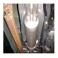
INSTALL MUFFLER # B ONTO HEADPIPE 1  $\frac{1}{2}$ " TO 2". USE CLAMP '# G TO SECURE MUFFLER TO HEADPIPE. DO NOT TIGHTEN. USE A JACK STAND TO HOLD UP THE MUFFLER. OUTLETS SHOULD BE LEVEL.
