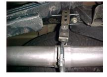
ON THE DRIVERS SIDE MEASURE APPROX. 17" FROM THE REAR OF THE FRAME USE THIS 1" HOLE TO BOLT HANGER # K USING THE TOP HOLE ON HANGER & HARDWARE PROVIDED, REPEAT FOR PASSENGER SIDE.
