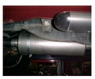
INSTALL MUFFLER # C ONTO YOUR RESONATOR#B 1 ½" –2". USE CLAMP # I TO SECURE MUFFLER TO THE PIPE, DO NOT TIGHTEN.
