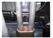
5. Install muffler #C onto headpipes 1.5"-2" with the louvers facing towards the converter. Use a jack stand to support the muffler. Use clamps #J to secure the muffler to the headpipes. Do not tighten. Muffler inlet is looking into the louvers.
