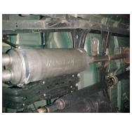
INSTALL MUFFLER #B ONTO THE HEAD PIPE 1-1/2" TO 2". OUTLETS SHOULD BE ON TOP. THEN INSTALL BAND CLAMP # H ONTO MUFFLER INSERT HANGERS INTO RUBBER GROMMETS.
