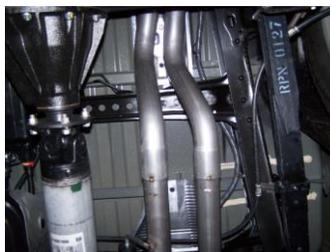
7. Install the passenger side overaxle tailpipe #F to the extension pipe 1.5"-2". Using clamp #I to secure pipes together. Do not tighten. Insert welded hanger into rubber grommet.
