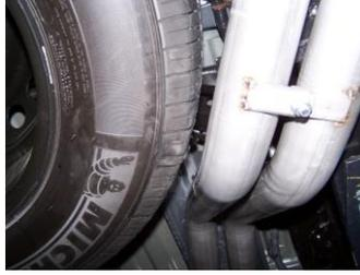
9. Use bolt kit #J to secure tabs. Make sure driver side tab is on the bottom. (You may need to loosen up the spare tire and move it over for better clearance.)
