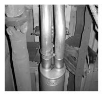
THEN, INSTALL DRIVERSIDE TAILPIPE #D. SUPPORT THE MUFFLER WITH A JACK STAND. THEN INSTALL PASSENGER SIDE OVERAXLE #C. INSERT WELDED HANGER ON TAILPIPE INTO FACTORY RUBBER GROMMENT.
