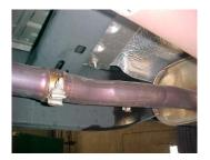
TO REMOVE YOUR STOCK EXHAUST, REMOVE IT FROM THE CLAMP LOCATED JUST IN FRONT OF THE MUFFLER REMOVE HANGERS FROM RUBBER GROMMETS BY PULLING EXHAUST TOWARDS THE REAR OF THE VEHICLE, USE WD-40 TO AID IN REMOVAL, LEAVE GROMMETS IN PLACE.
